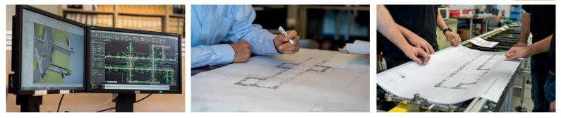
The LOGO!MAT Planning Tool is specially tailored to LOGO!MAT Conveyor Systems and includes drawing blocks of all our standard components. The tool enables customers to quickly design and develop a layout of their assembly line using a standard CAD program. The system can be built as planned because the planning blocks factor in spacing and other requirements for LOGO!MAT Systems.
