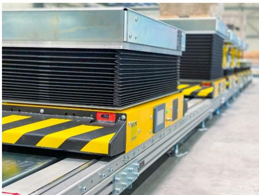
The new LOGO!MAT Scissor Lift is an integrated lifting platform with a stroke of up to 300 mm. The applications and benefits of the Scissor Lift go far beyond the ability to position your part at an ergonomic height for each of your operators. The Scissor Lift can be also used to place parts on an external structure with indexing points for precise positioning or force absorption in automatic stations. This eliminates the need for expensive floor excavation and reinforcement.
